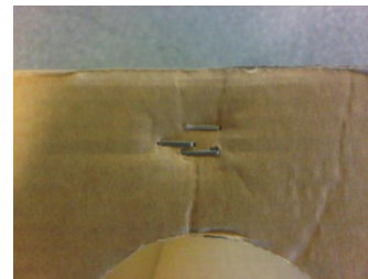
Example of insufficient stapling
