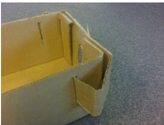
Folding construction without the use of glue or staples
