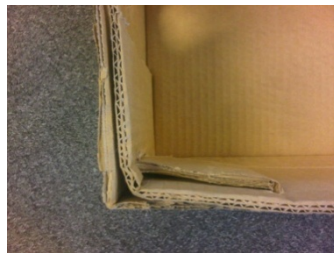
Folding construction without the use of glue or staples
