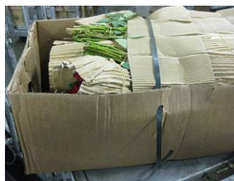
Strapping to prevent sliding in box
